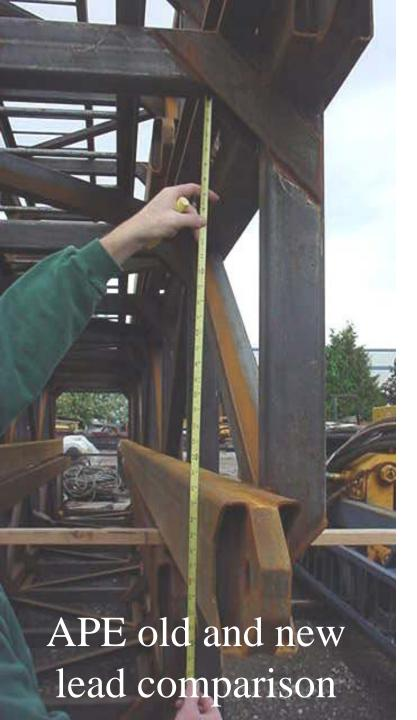
The old style **APE 32** inch lead in on the right. The new style lead shown on the left is deeper.
